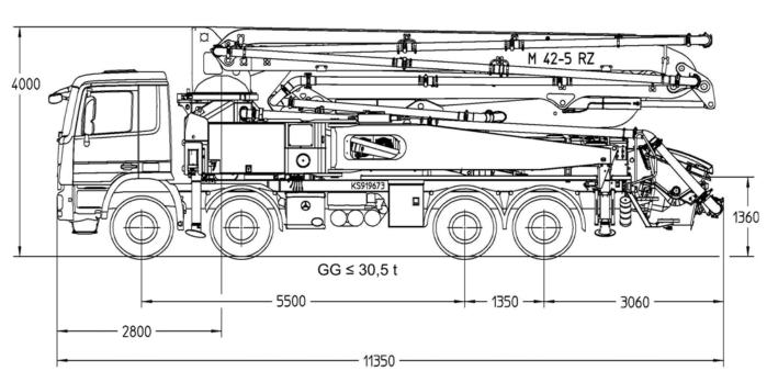
Note: Standard version. Dimensions and weights depend on truck, pump model and equipment. Dimensions in mm, MB-Actros 3241, Euro 5 as example. For illustration only.
